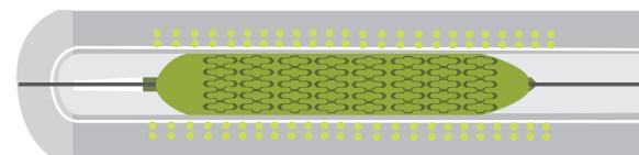
**Step 2:** Drug release from stent and parts of balloon upon expansion
