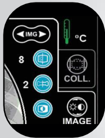
Real-Time Image Management Access to image improvement features ie: Noise Reduction, Edge enhancement, Image Rotation, Image Inversion & Reference Image
