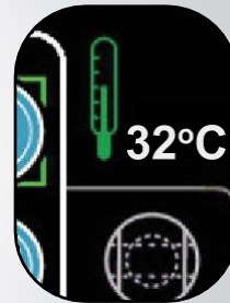
Real-Time Heat Monitoring The Technician can visualise monoblock thermal status in real-time on the Touch panel
