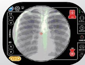
Laser Aimer Pointer display on live / LIH Image For radiation free positioning
