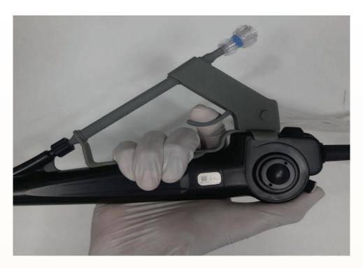
Irrigation Mode (Trigger released) Default Mode
